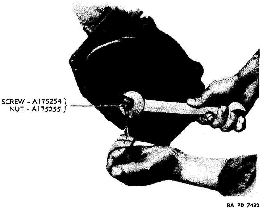
Figure 161—Steering Gear Lever Shaft End Play Adjustment
