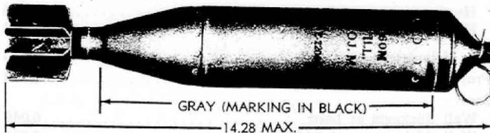
SHELL, ILLUMINATING, M83, W/FUZE, TIME (FIXED), M65; 60-MM MORTARS, M1 AND M2, COMPLETE ROUND
