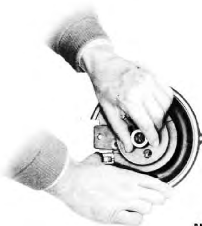
Figure 89 – Engaging Rack to Ratchet Segment
