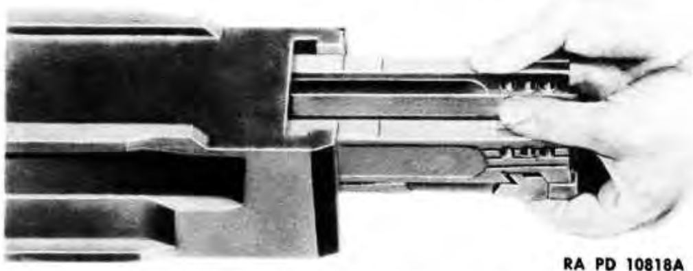
Figure 76 – Removing (or Replacing) the Breechblock
