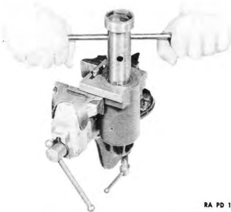
Figure 71 – Unscrewing the Rear Buffer Sleeve
