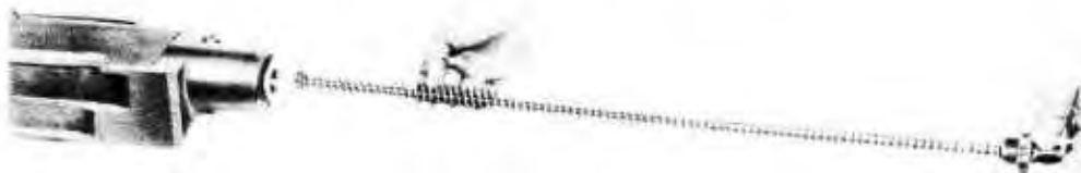
Figure 83 – Inserting the Driving Spring Group
