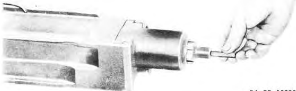
Figure 69 — Inserting the Driving Spring Assembling Tool
