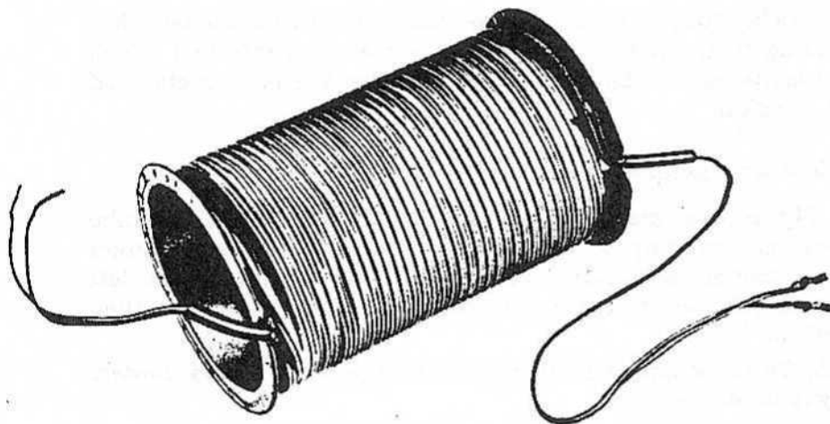
Figure 42—Rear Spacer Tube Wound With Wire
