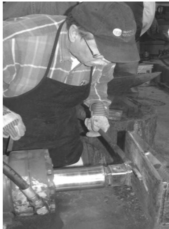
Parks Low using the hydraulic press to shape the welded cable.
