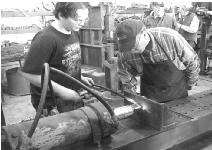
Consolidating the weld with a hydraulic press
