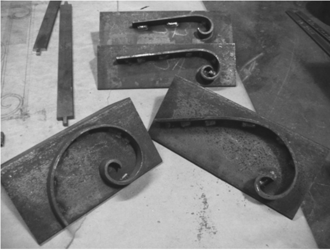
The Jigs. Notice the Tenons On the Ends of the Frame Pieces (upper left)
