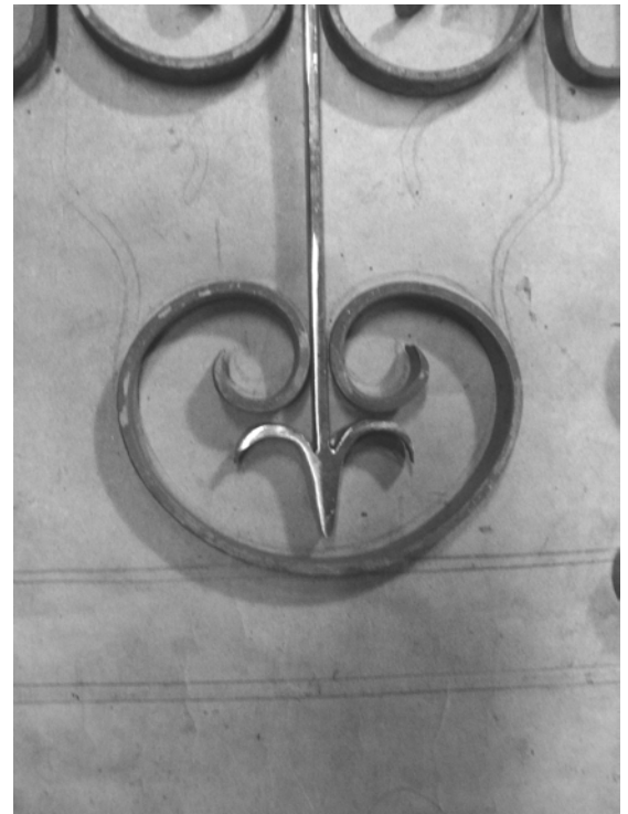
Assembly On the Brown Paper Master Drawing
