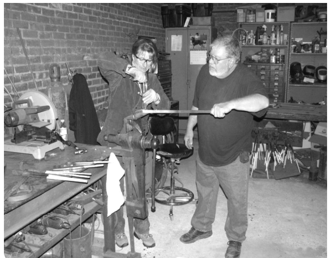
Jim Alexander and Jackie MacCleod demonstrate using a jig to make one of many scrolls
