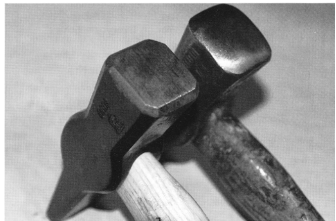
The left hammer is new, the right is dressed
