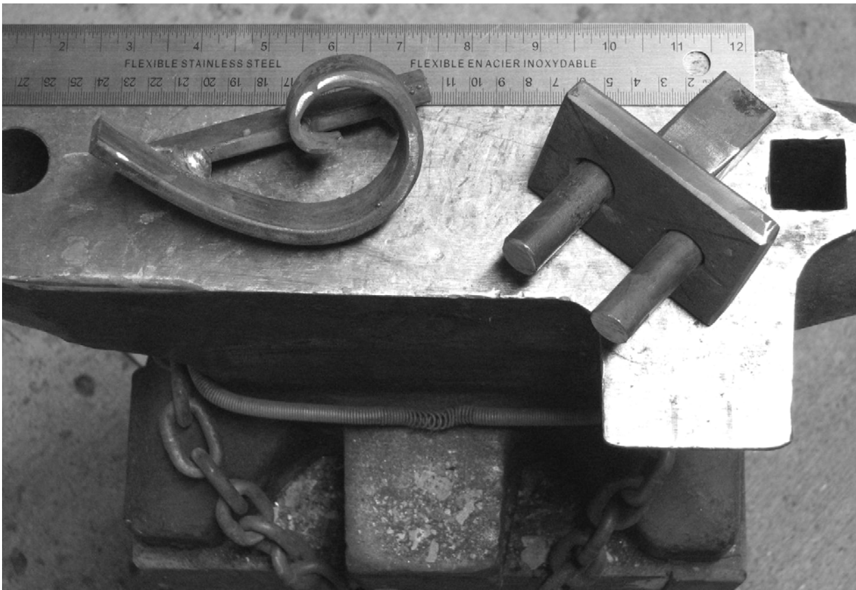
Scrolling jig and bending tool made at the meeting.
