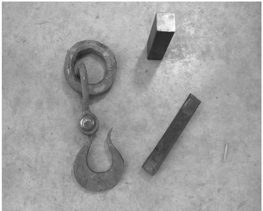
Hook made by Tom on power hammer. Starting stock on right.
