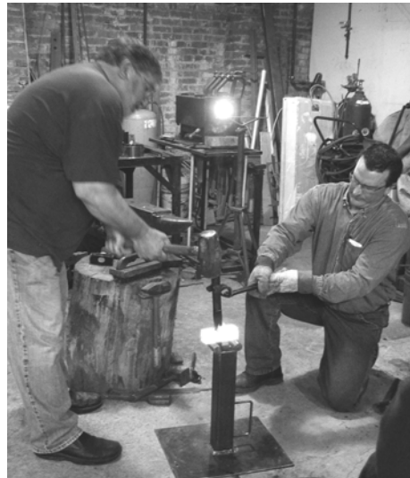
Jimmy Alexander Striking for Jim Kennady forging nail header (left) and hammer head (right)
