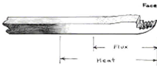
Figure 9: Fluxed face heated from below.
