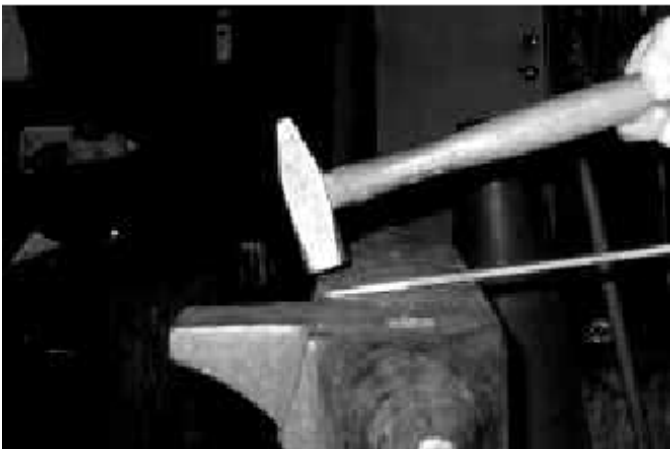
5. Correct position of the bar on the anvil to finish the ribbon taper. Notice that the bar is slightly elevated on the holding end. Note also the angle of the hammer.
