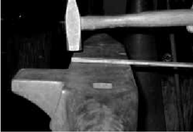
4. Correct position of the bar and set-up shape on the anvil to begin drawing out the ribbon taper.
