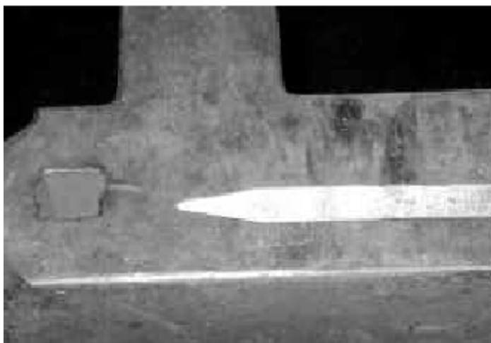
3a. Top view of the set-up shape. Notice that the width of the parent stock has decreased towards the tip.
