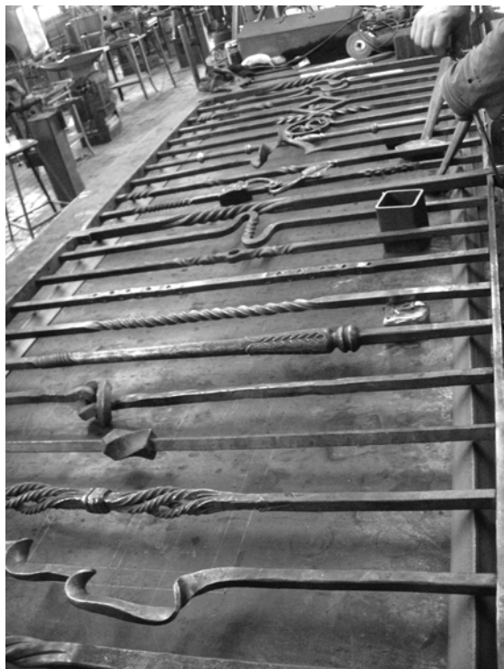
Assembling The Railing
