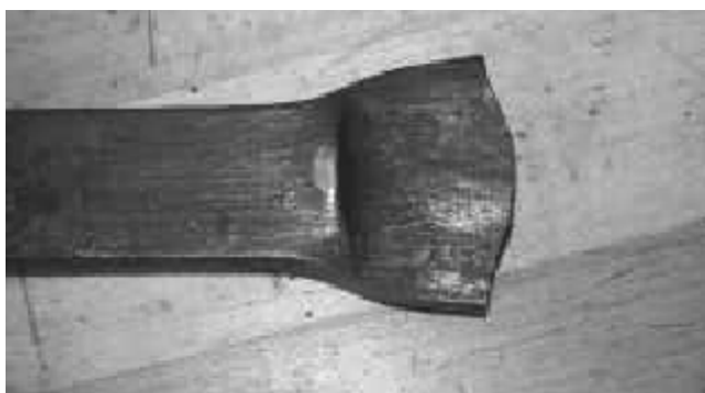
Fig. 11. Bottom of bar showing transition made by rounded corner of the anvil.
