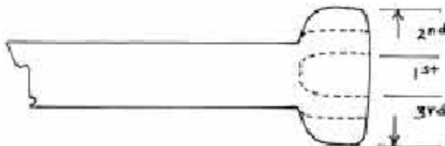
Fig. 12. Work the middle, then the side furthest from you, then the side nearest you.
