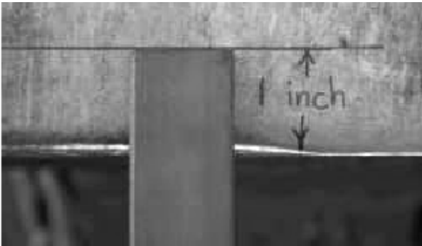
Fig. 5. One inch of the bar on the anvil face.
