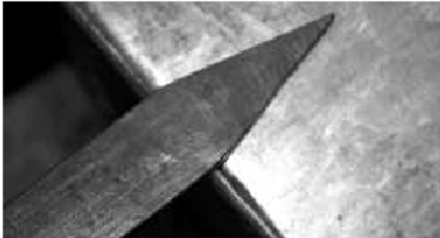
Fig. 21. Place just the set-up flat on the anvil face.
