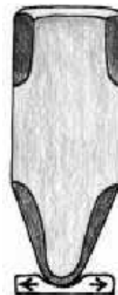
Fig. 4. Peen pushes metal to either side.
