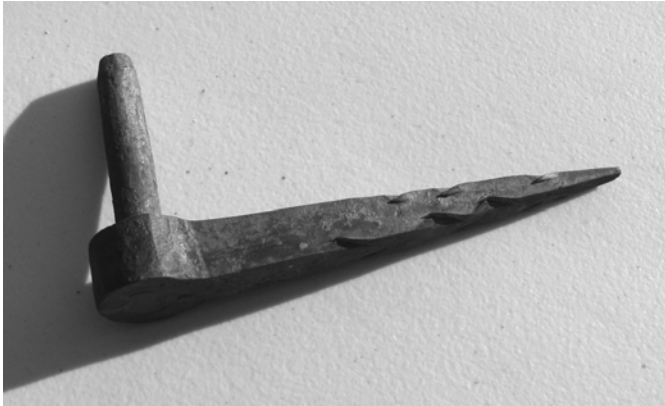
Two Piece Forge Welded Pintle
