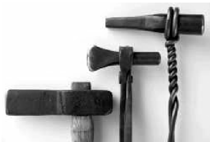
8. A wooden-handled chisel, left, dedicated chisel-holding tongs, center, and a wrapped handle (on a punch), right.
