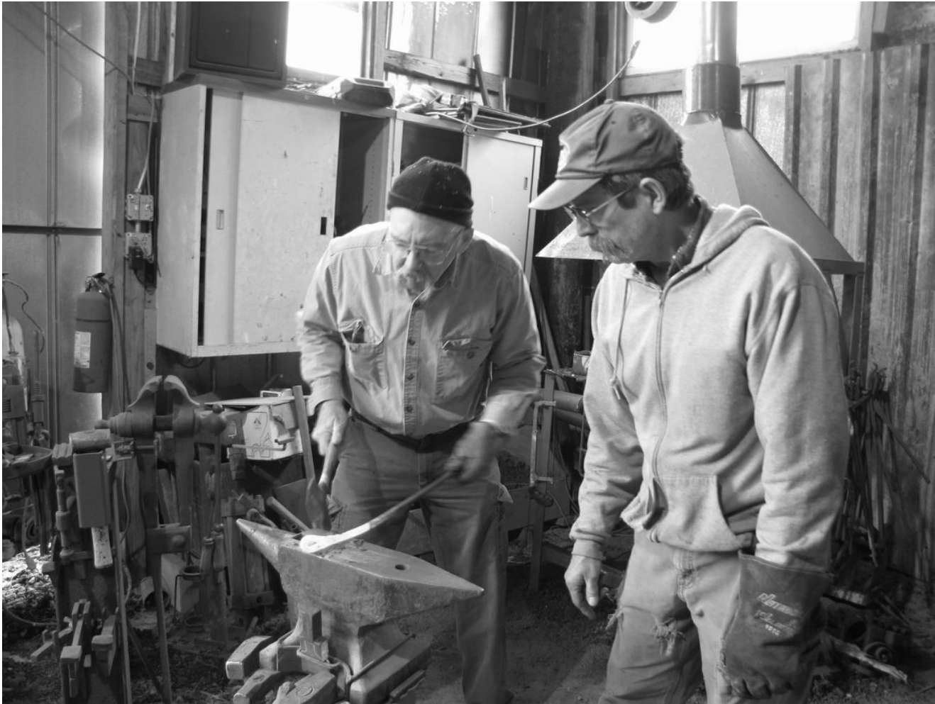
Robert Temberlake observing as workshop Walt Beckweth works on forge welding.
