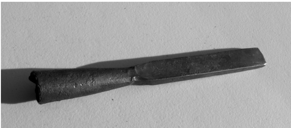
Socketed Wrought Iron Chisel With Steel End
