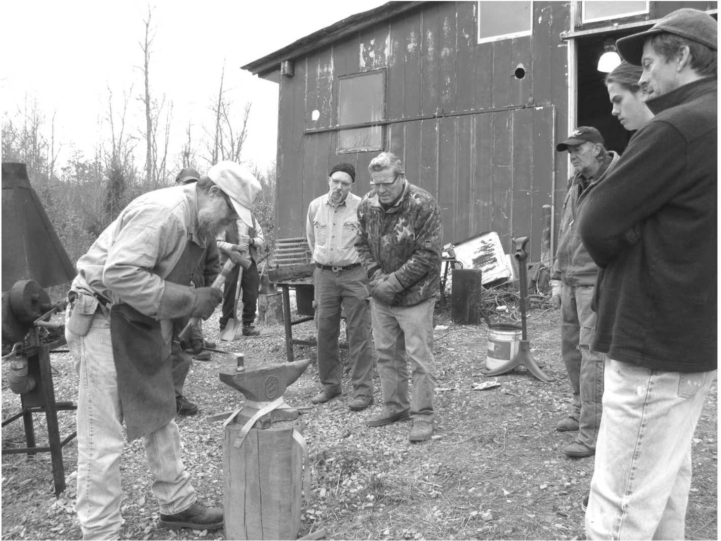
John Fluke demonstrates cutting the bar prior to folding and welding it
