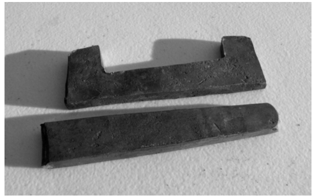
New Forged Parts For the Vice.
