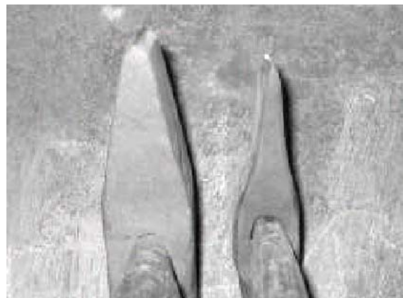
3. Notice the difference in the thickness between the cold cut (left) and the hot cut (right).
