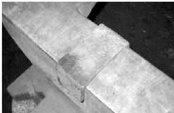
9. This cutting saddle was made from 1/2" x 3", lies flat on the anvil face and fits snugly over the edges. The thickness has been reduced by re-dressing the surface to eliminate surface scars made from cutting through the workpiece. "blacksmith's helper so the workpiece lies flat on the anvil or cutting saddle.
