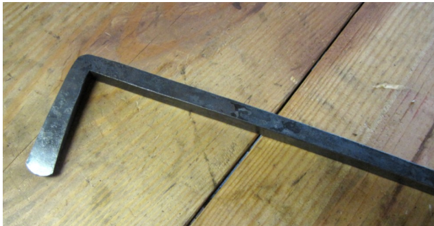
Spike Dog . Note the 90 Degree Twist Between the Two Ends
