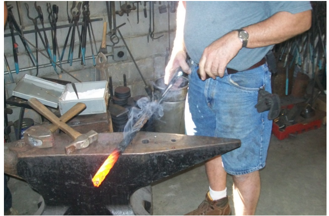
Butch Silver Forging on a Cable Damascus Billet
