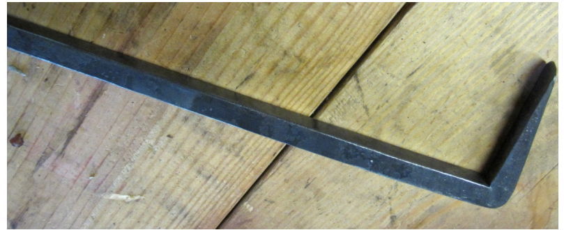
Spike Dog . Note the 90 Degree Twist Between the Two Ends
