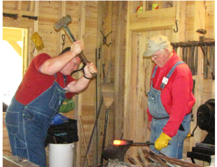
Lenny Moore and Don Forging an Eye in a Chisel
