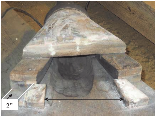
Small 1/2" thick pieces of wood that help hold the floating arms in place with the aid of a strip of leather that is tacked to them and the floating arms.
