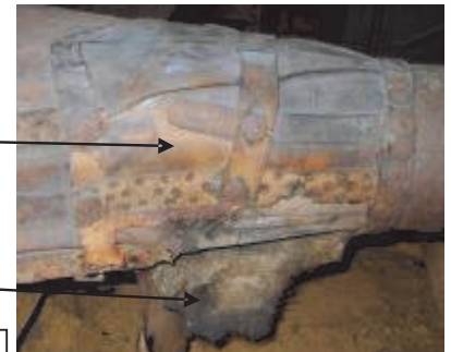
This is a photo of another piece of a very old smaller rotten bellows that I have. Note the wood shims and how the other pieces are made.
