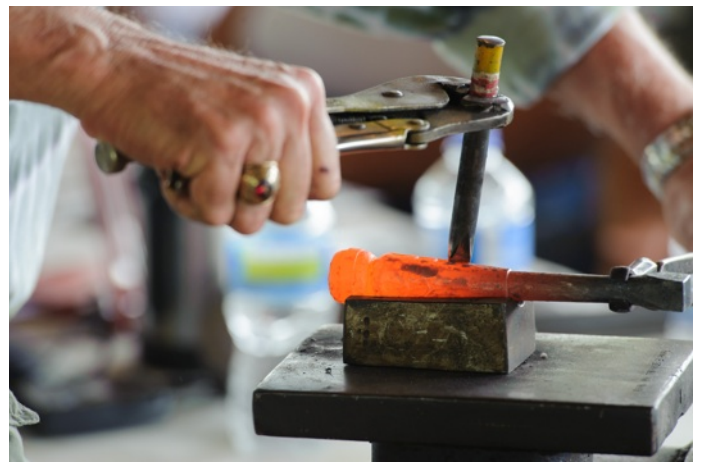
The X for the design being punched into the hot preform. Note the tapered round bottom swage supporting the piece.
