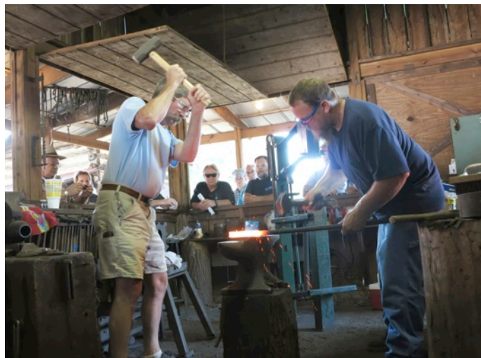
Robert Timberlake (L) and Joe Allen (R) forge weld the billet
