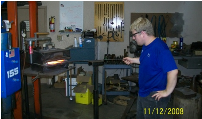
Shawn Emmons forges a knife from an engine head bolt
