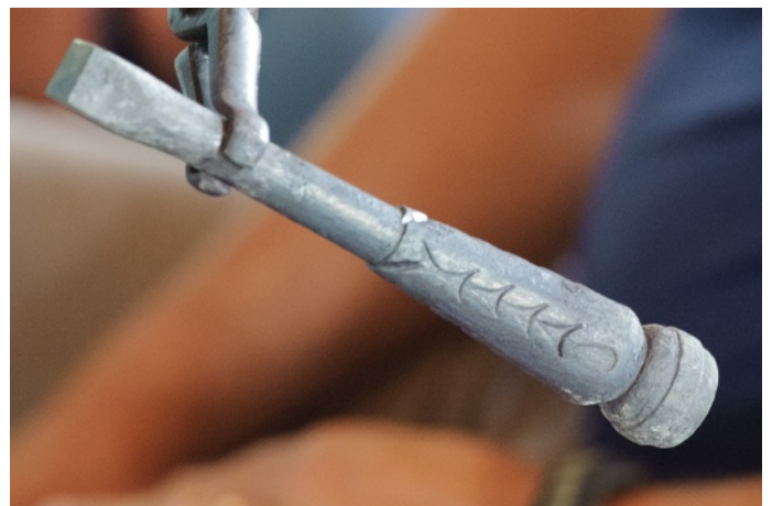
Preform after chiseling hot with multiple passes of the X and teardrop shape.
