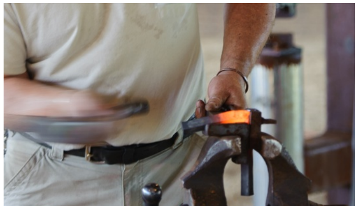
Upsetting the corner in the vise against a v-block.
