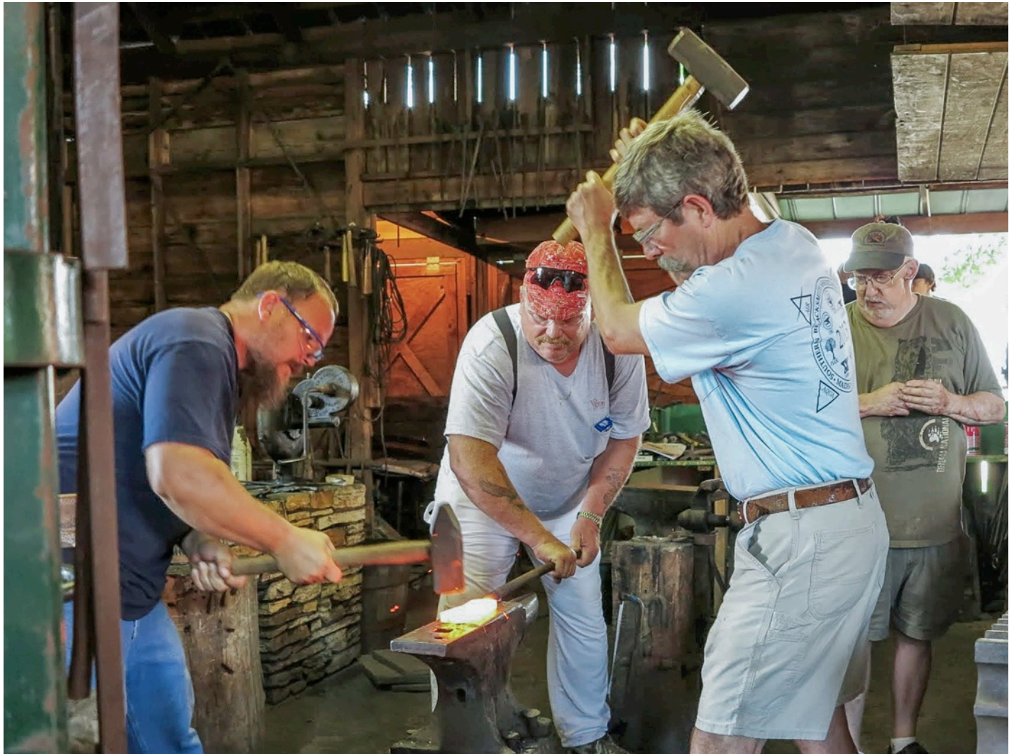
Joe Allen (left), Don McDunnah, and Robert Timberlake forge welding a damascus billet under the watchful eye of Master Bladesmith Tommy McNabb (right)
