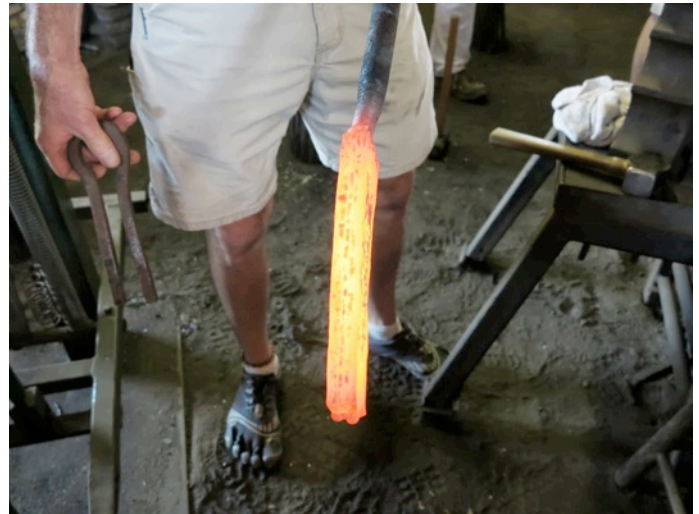
The billet is drawn out to twice its original length
