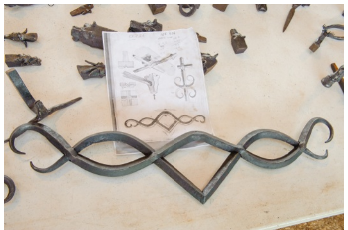
A finished piece showing use of a square corner on the diagonal
