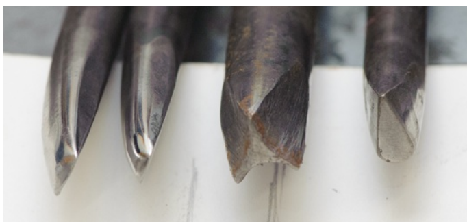
The chasing tools used to create the leaf (1/8 x 1/4 rectangular punch not shown)
