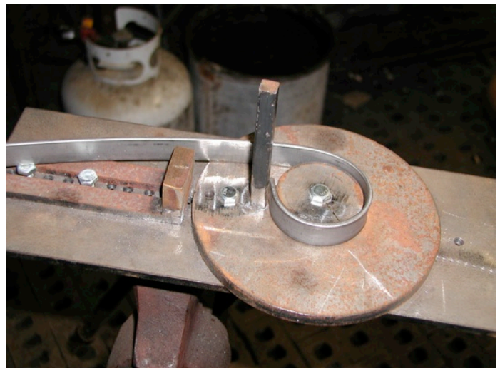
Cold bending jig used to make simple scrolls
