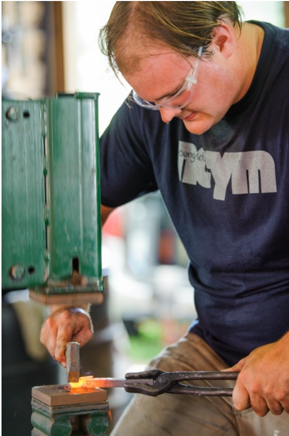
Using a self-made set hammer to flatten a bald headed wizard
