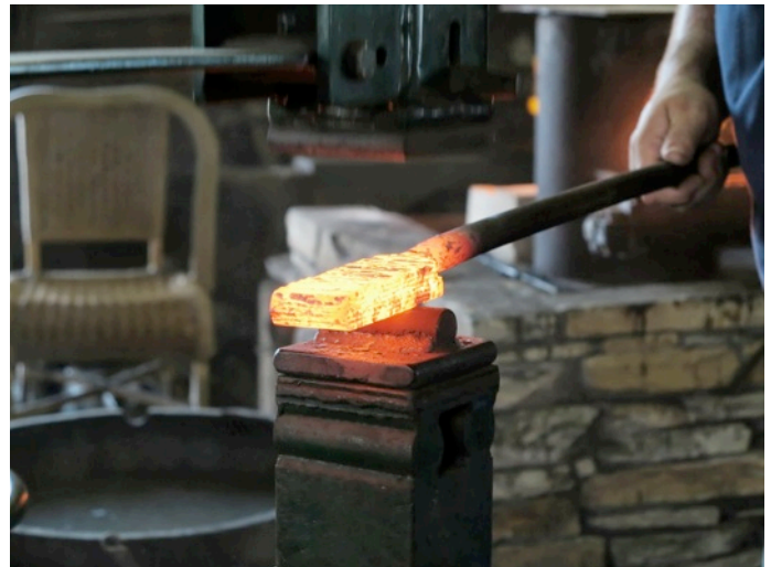
The long billet is cut, folded and forge welded again to double the number of layers
