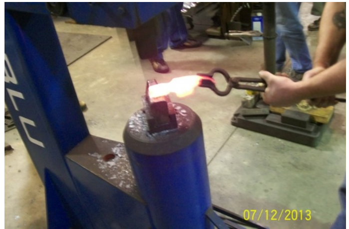
Forging a hawk from a carpenter's hammer
