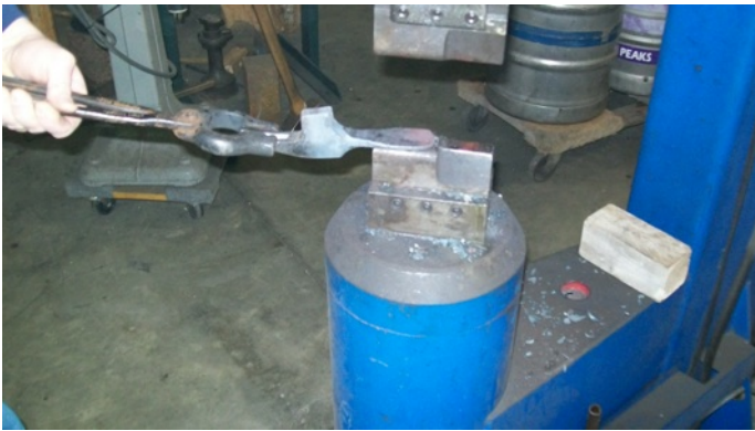
Brian Swink forging an adz from a carpenter's hammer. The claws form a convenient handle and keeps the socket from being deformed.
