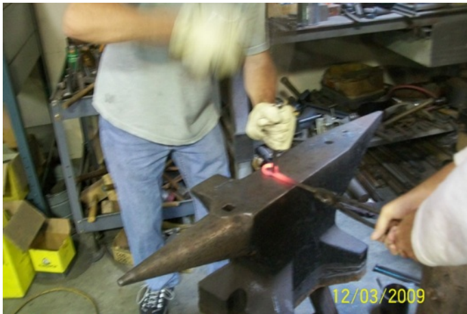
Dave Stitt forges a bottle opener from an open end wrench
