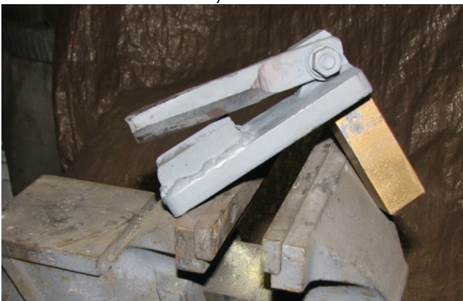
Side view of the tool showing the hardie post.
