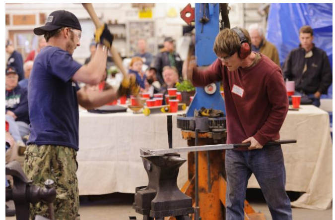
Driving a drift to open the slit hole in the bar
