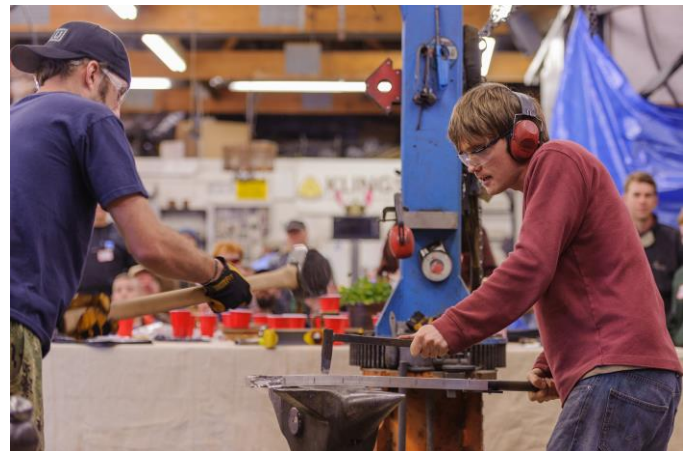
Slitting a hole in the bar, Matt Clark striking
