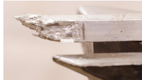
The result of forging an overheated aluminum bar
