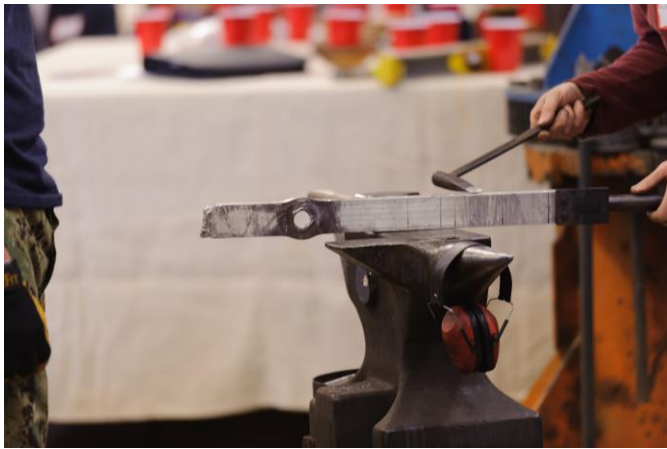
Finished slit and drifted hole
