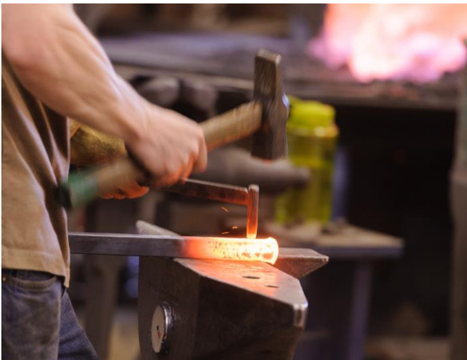
Marking to punch a hole
