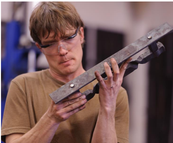
The tenons are cut to length and fit
