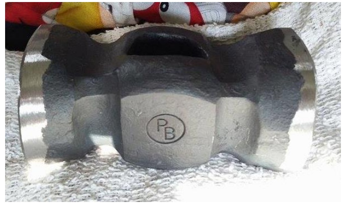
Stamping your touchmark into a product is what separates a hobbyist blacksmith from a professional.
