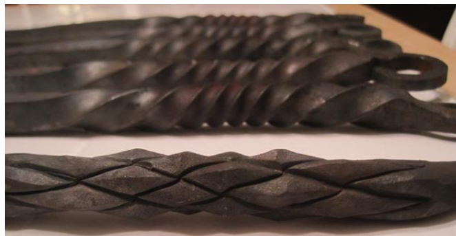
Above is a detailed picture of the handles. Check out the pineapple twist!
