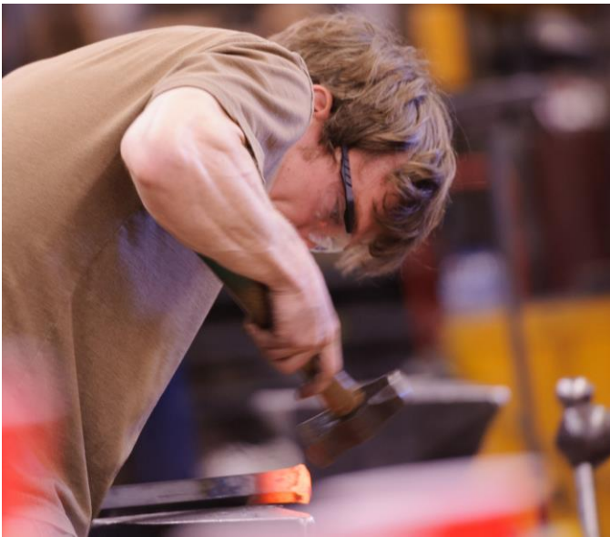
Finishing the flare on the upset with the hammer
