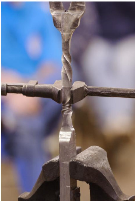
Reaching the limits of a tight twist in aluminum
