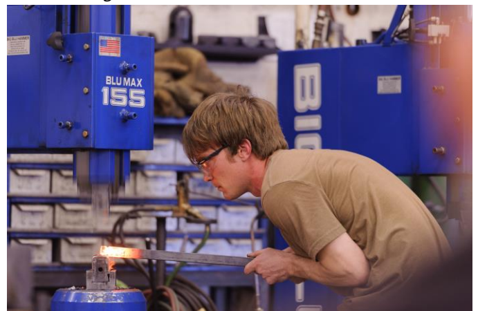
Drawing out the tenon on the power hammer
