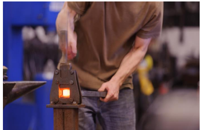
Smithin' Magician with butchers was used to isolate a tenon
