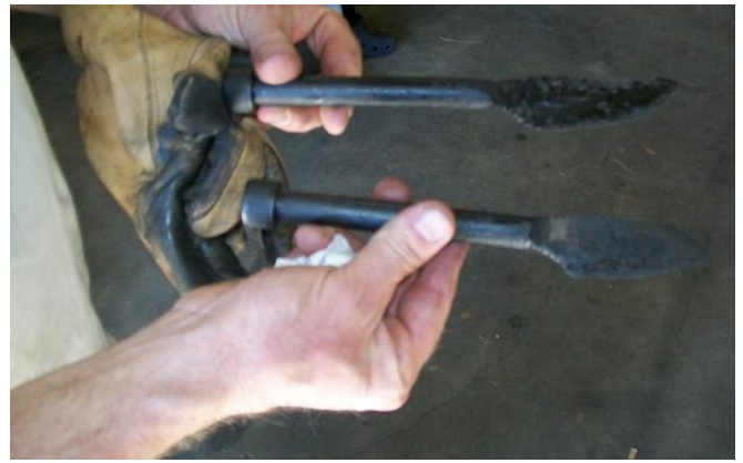
This smith used old bolts to forge knives.
