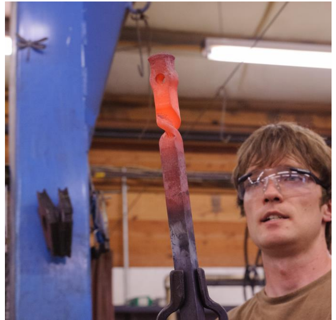
The bar has been flattened and then twisted a quarter turn
