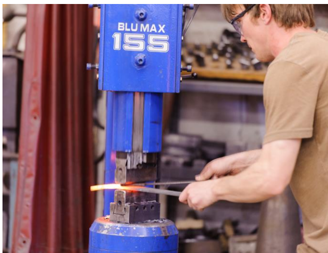
The backplate of 1/8" steel is textured
