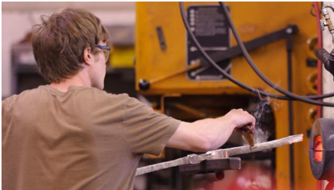
Lucas tests temperature of aluminum with a pine stick
