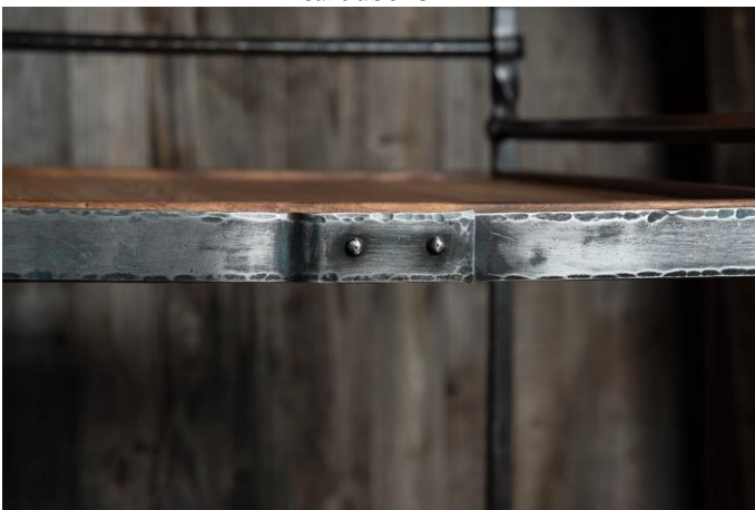
Check out these textured trim pieces. Texturing is one of the best ways to move beyond beginner smith and into the realm of journeyman.
