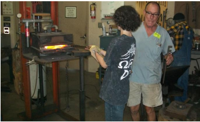
Heating up the spring and getting the bending fork ready
