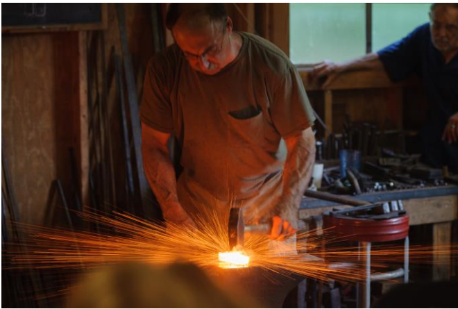
Nothing like a good forge weld.
