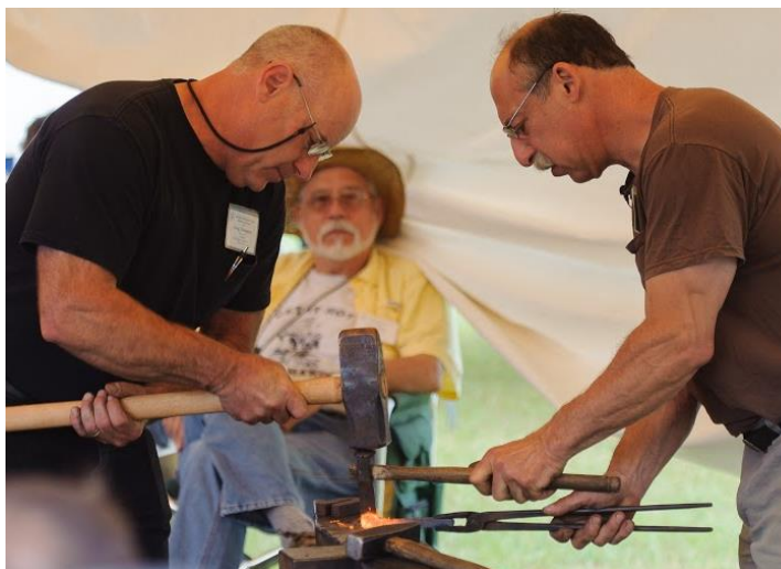
Peter Ross working with a striker to cut the slot for the compass pivot.
