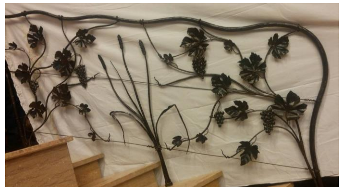
While many parts of this railing were forged, Stefano has integrated cast pieces to add weight to the flowers. The flow of the top member is particularly natural in this railing.
