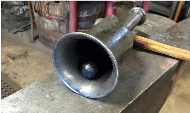
Not all of Tom's pieces are made from solid steel as illustrated above with this bell, currently in the process of being forged. Below is the finished product.
