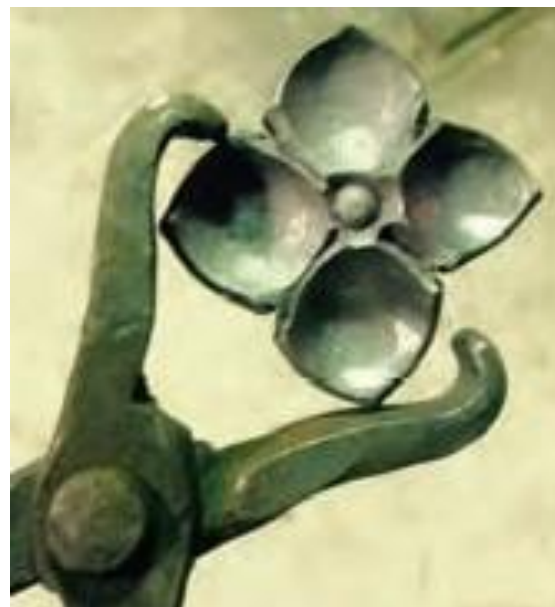
Use a ball fuller to move the material on the petals in place.
