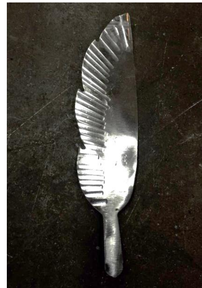
Feather made by Oak Hill Iron. Also a good use for a treadle hammer as long as you have steady hands (& feet).
