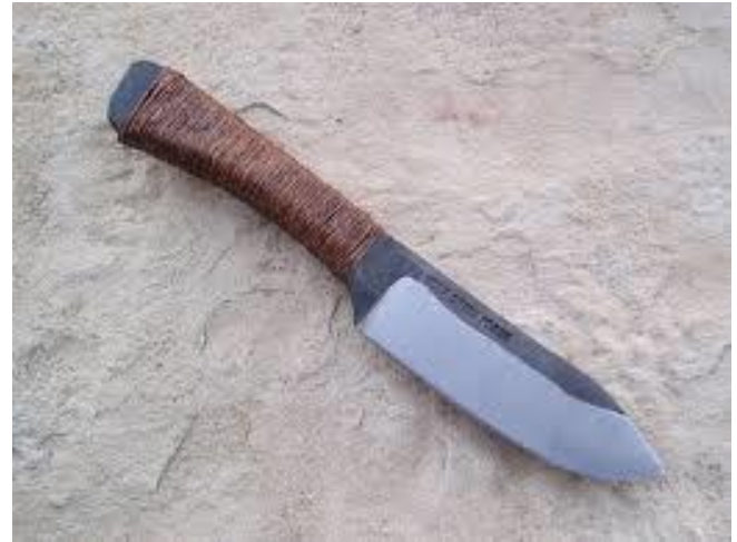
Knife made by Wolf Creek Forge out of L6.
