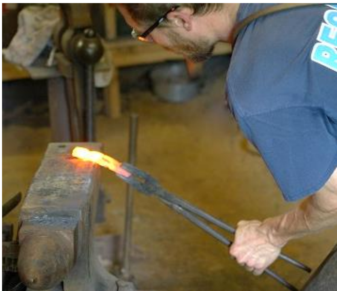
Using the marks as guides the eye is set down.
