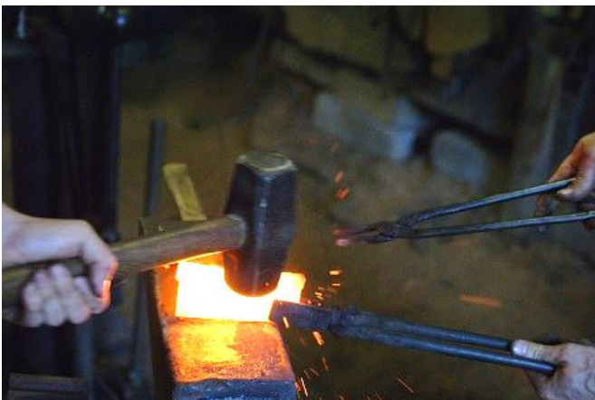
The steel is welded to one of the two pieces of wrought iron.
