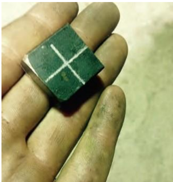
Mark the square into 4 smaller squares with a piece of soapstone.
