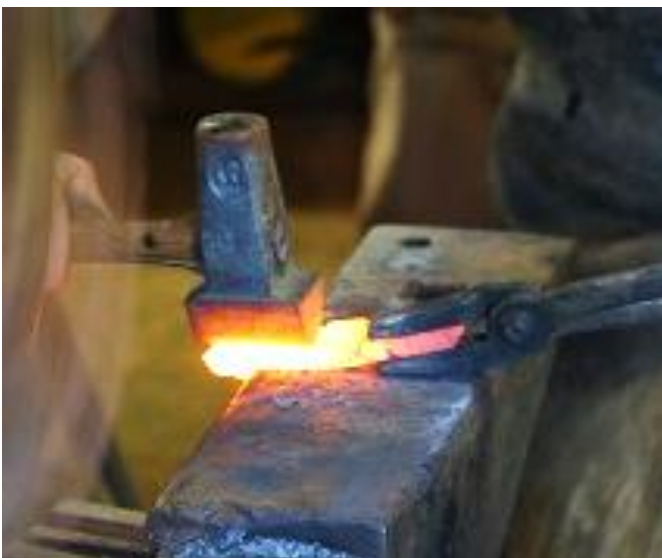
A top fuller is used to spread what will become the "ears" or "lugs" of the eye.
