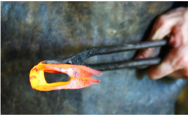
Edge view of the eye after folding. Notice the scarfs.
