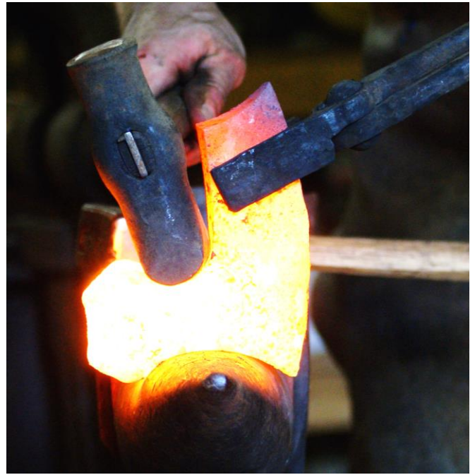
The horn of the anvil and a large top fuller are used to profile the joint between eye and blade.
