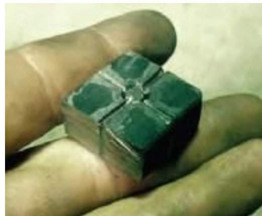
A circular punch like an eye punch can make the center mark and a straight-edged chisel for the lines.
