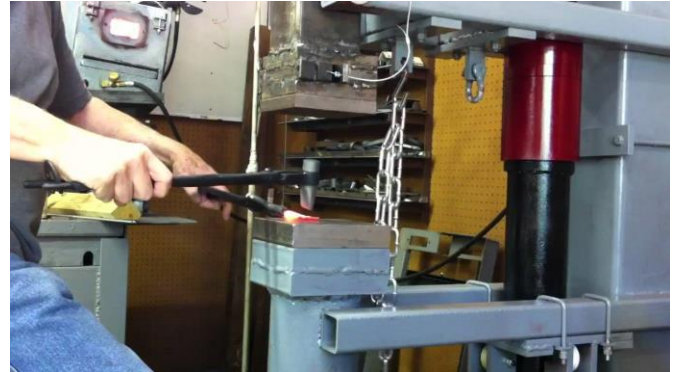
Treadle hammer in use with fulling tools
