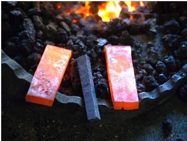
The raw material. Two pieces of wrought iron, \frac{3}{8} " x 5"; and one piece of steel, \frac{3}{8} " square x 5". One piece of wrought iron will become the eye, the other along with the steel will become the blade.
