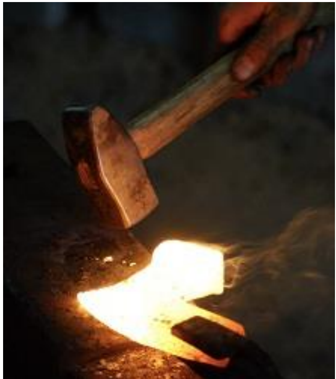
The eye and blade are welded together.
