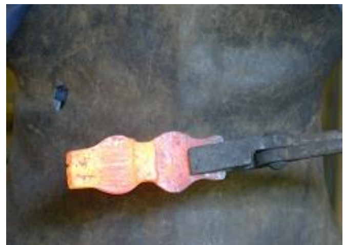
Outside view of the eye. The raised section in the middle is the poll.
