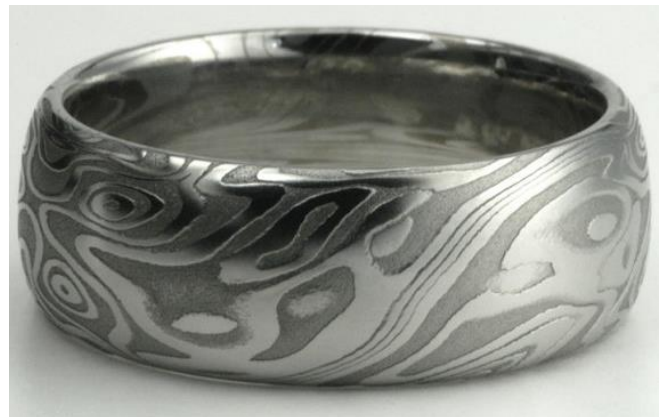
Ring made with Damascus. Note the shininess of the L6 in it.
