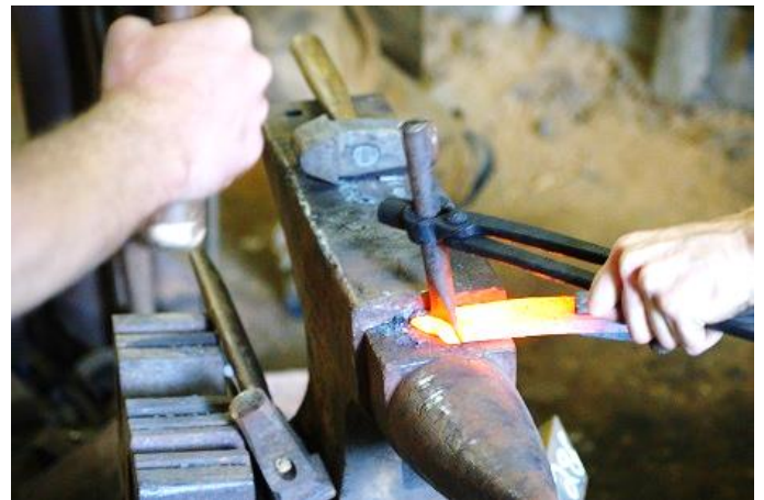
The blade is trimmed with a curved chisel.
