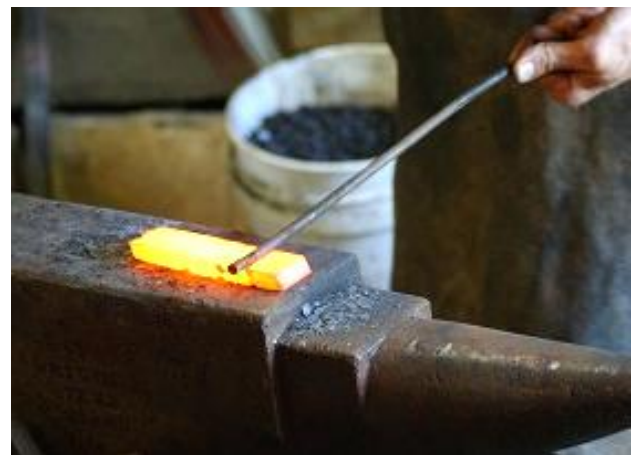
Moving to the second piece of wrought iron, a small round rod is used to mark the location of the poll and the extent of either side of the eye.
