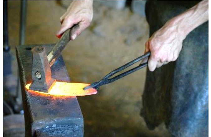
After drawing out the cutting edge, the blade is smoothed with a flatter.
