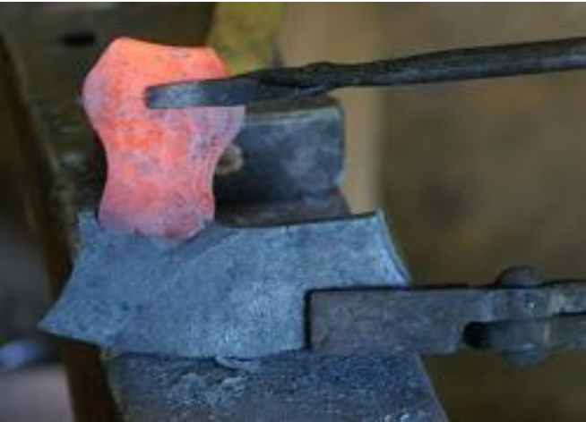
The eye sandwiches a scarf on the upper back side of the blade.
