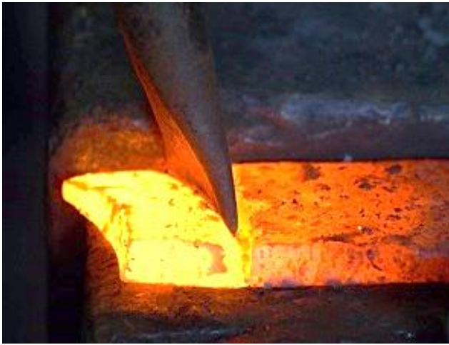
The lower end of the blade known as the "beard" is trimmed to length with a curved chisel.
