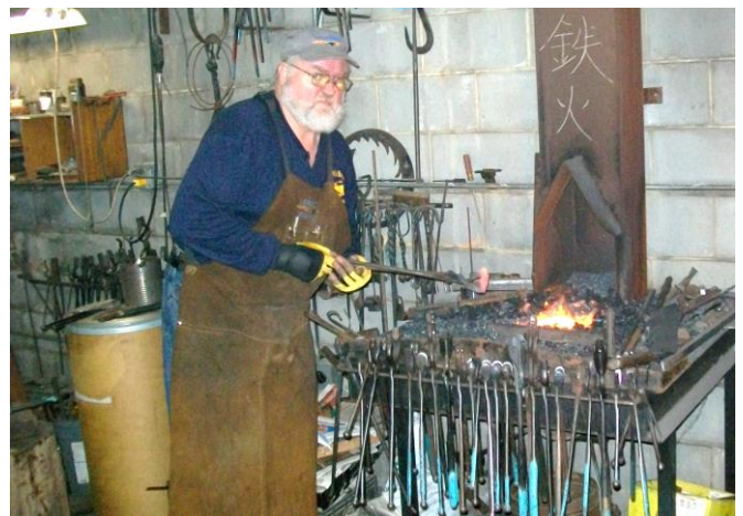
James "Jeep" Sabo working on reforging some worn rock hammers that need to be lengthened
