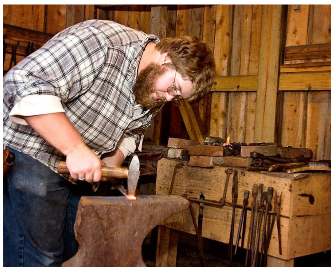
This volunteer is Kevin and he is forging a knife blade as a demonstration.
