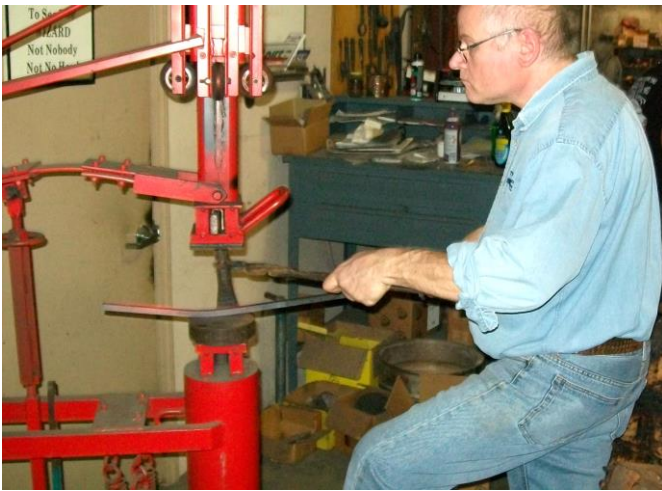
Matt Ballent using the treadle hammer to forge grooves in a project. Treadle hammer does not get much usage at our meetings - good to see someone using it.
