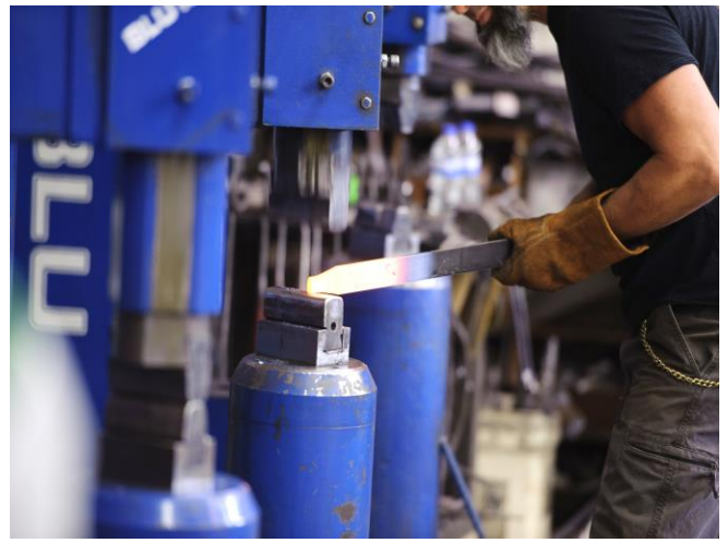
Jason roughs in the profile of the blade on the power hammer
