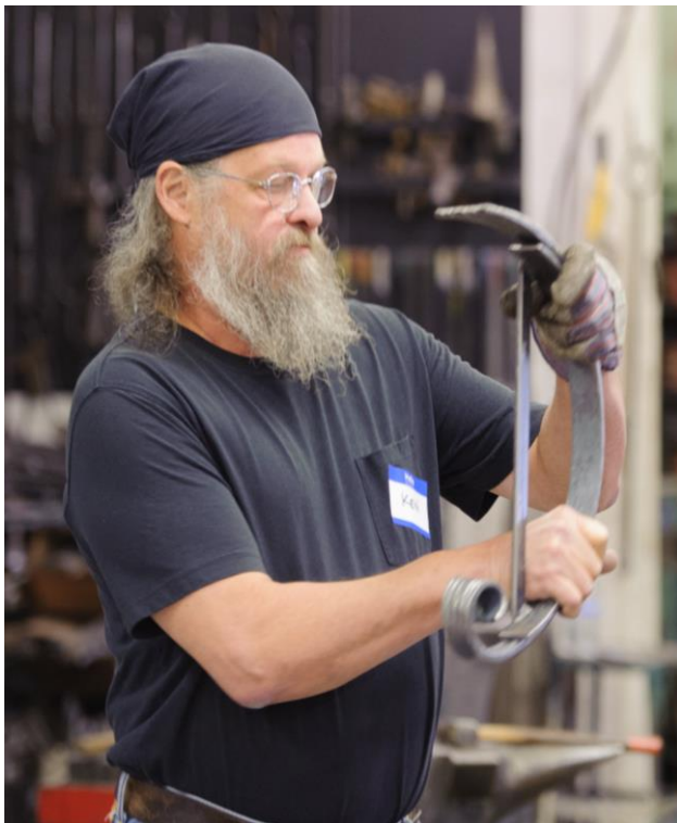
Ken Thomas & a complete table leg with a jig for bending it
