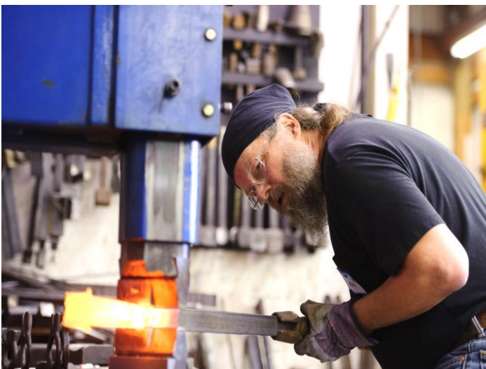
Tapering the leg under a Big Blu power hammer
