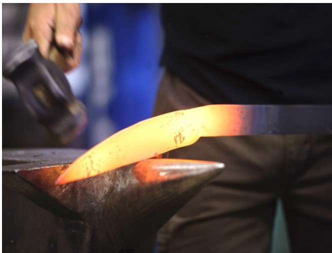
Pre-curling the blade before drawing out the cutting edge
