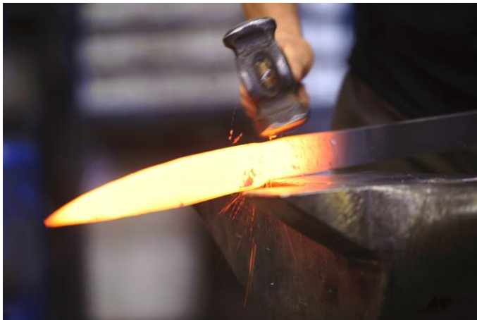
Setting down the handle with half-on blows on the anvil
