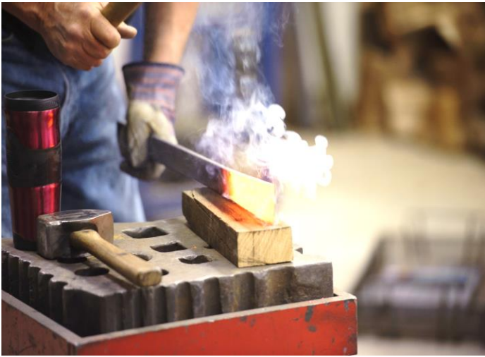
Straightening on a wood block
