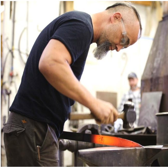
...and back and forth between anvil and power hammer to refine the profile
