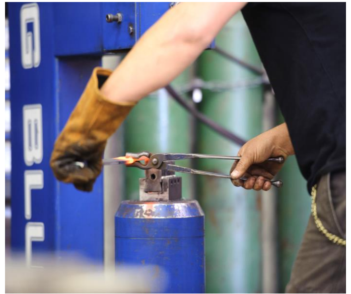
Drawing out the cutting edge under the Big Blu
