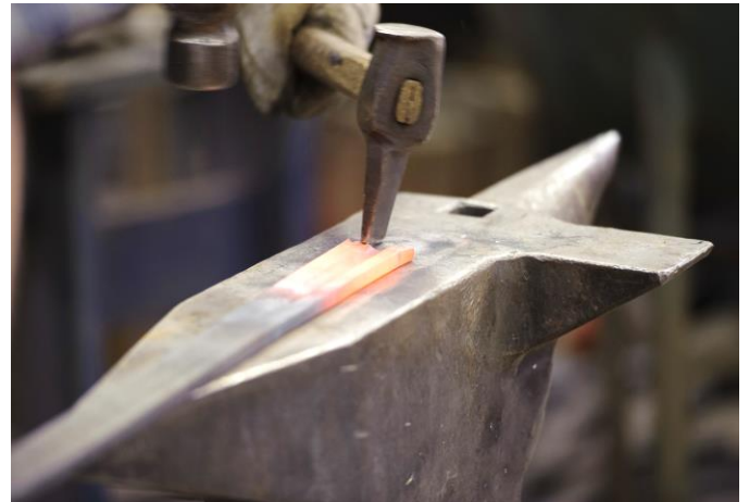
Hot chiseling two grooves on each edge
