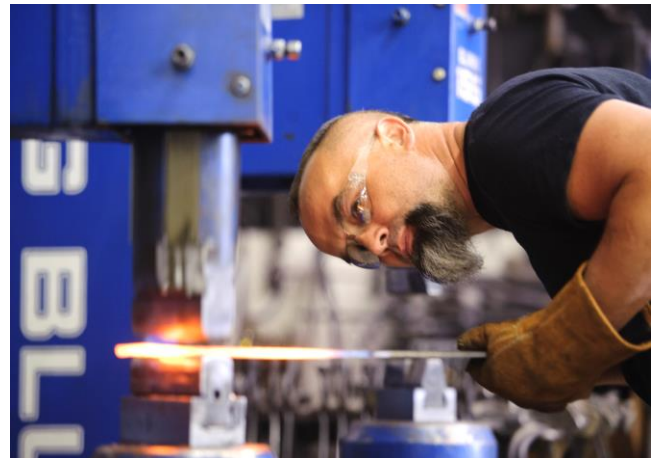
Flattening and forming a distal taper
