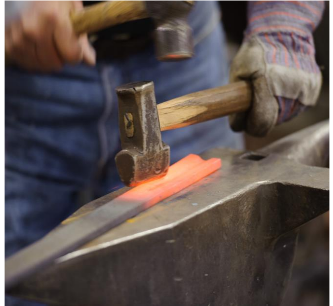
Completed fullered groove
