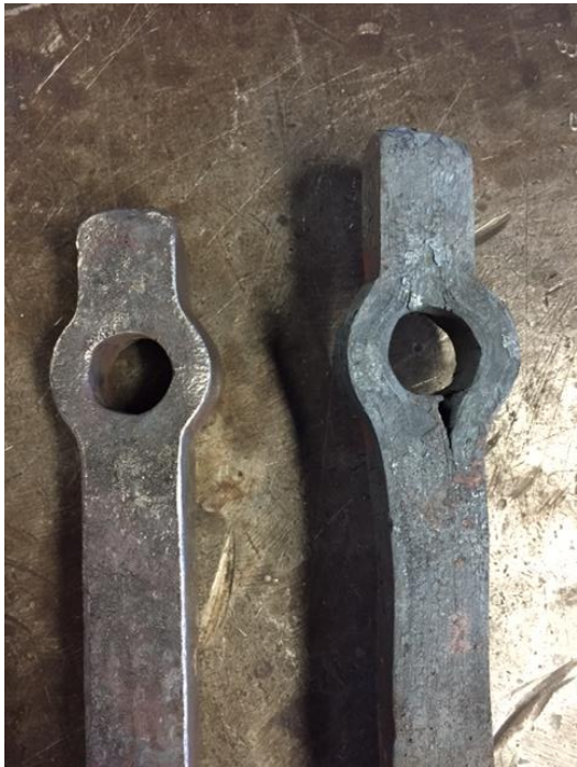
High quality wrought iron bolts at left Unrefined iron on right
