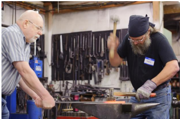
Chuck Brady assists as Ken forges a central fuller
