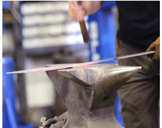
Refining the edge on the anvil; note the distal taper
