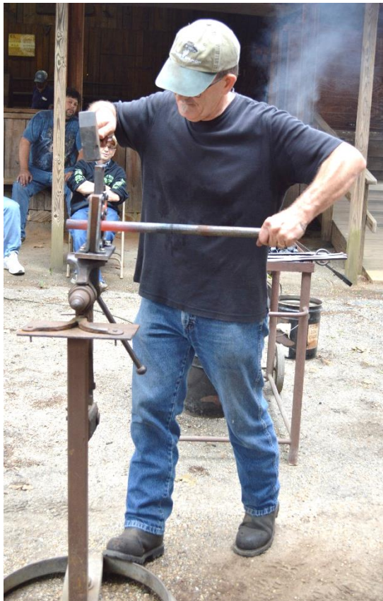
Paul Spainhour using a guillotine-style blacksmithing tool to work on his forgings. It was affectionately dubbed a Smithin'-magician by Keith Roberts.
