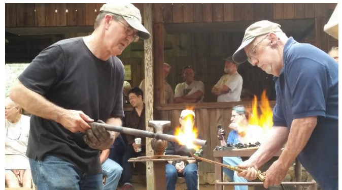
Paul used an oxy-acetylene set up to localize the heat.
