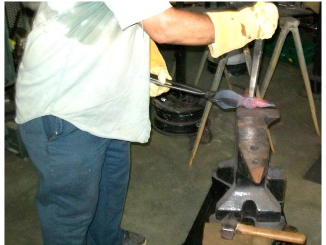
Denny Maloney forging a tomahawk from a ball pein hammer
