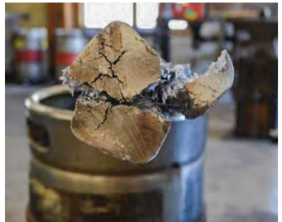
Figure 3: 3" Aluminum rod forged at too high a temperature
